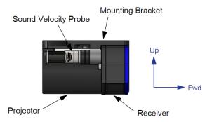
The sensors must be mounted rigidly and free from vibration, and there must be no independent movement between sensors. For Baywei M7, the GNSS antennas must have a clear sky view. It is recommended to separate the GNSS antennas by a distance of 2m.
